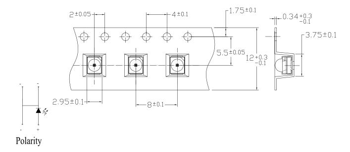
**Note:** Tolerances Unless Dimension  $\pm 0.1$ mm Unit = mm
